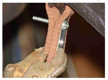
strap/plates going the wrong direction. Once you remove the bolt, in order to get the rivet in place you may have to use an electric drill to clean the hole out. If so, select a drill bit the same diameter as the rivet and be careful not to enlarge the holes in the rivet plates. Also, when you put the vise grips in place you need to make certain that you leave enough room so that the riveting tool can be placed on the rivet head with no interference.
