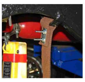
bolts in place and tightened, clamp the strap and rivet plates with some vice grips—in this picture you see the vice grips in place, the bottom bolt removed and a rivet inserted so that you can see how far it protrudes — for the picture I have the rivet through the
